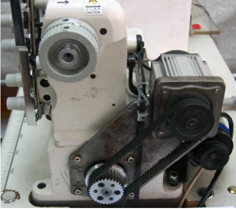
Fig.3.3 Illustration drawing of installation for back-mounted interlock sewing machine applicable for ASB50 control system
