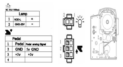
Fig. 4-1 controller link
