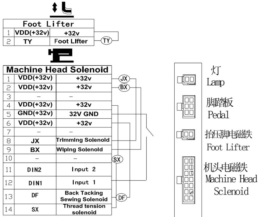
Fig. 4-1 controller link
